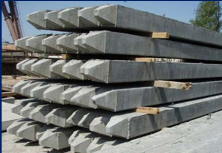
Pre-cast concrete piles
